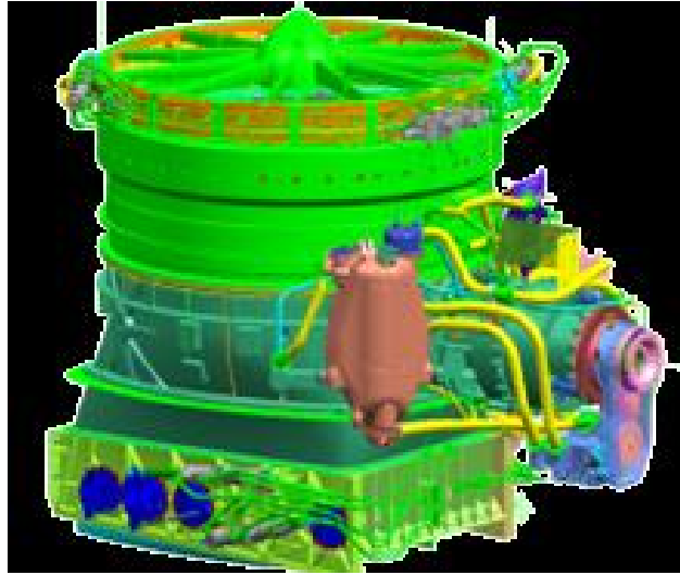
Figure A.2: Example CAD Geometry of the Liftfan for the USAF F-35B
